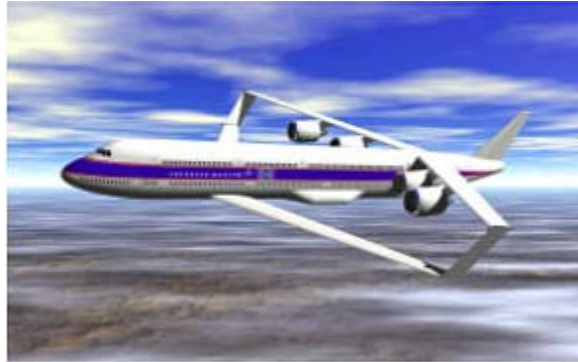
Figure-5: Lockheed-Martin box-wing freighter design
