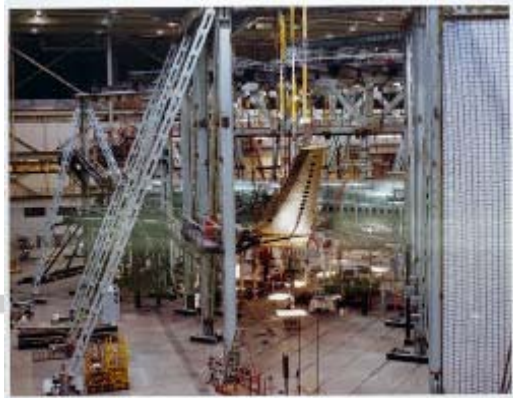
Figure-18: Static load test - Boeing 767
